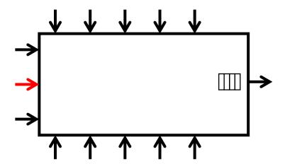
Assuming that all input ports are configured the same, and all are configured the same as the output port, we can observe that not all input ports can deliver a max size burst from the transmitting device; if they did, their combined data rates would be (in the above example) 13 times the data rate of the output port, and this is not allowed by the reservation protocol.
