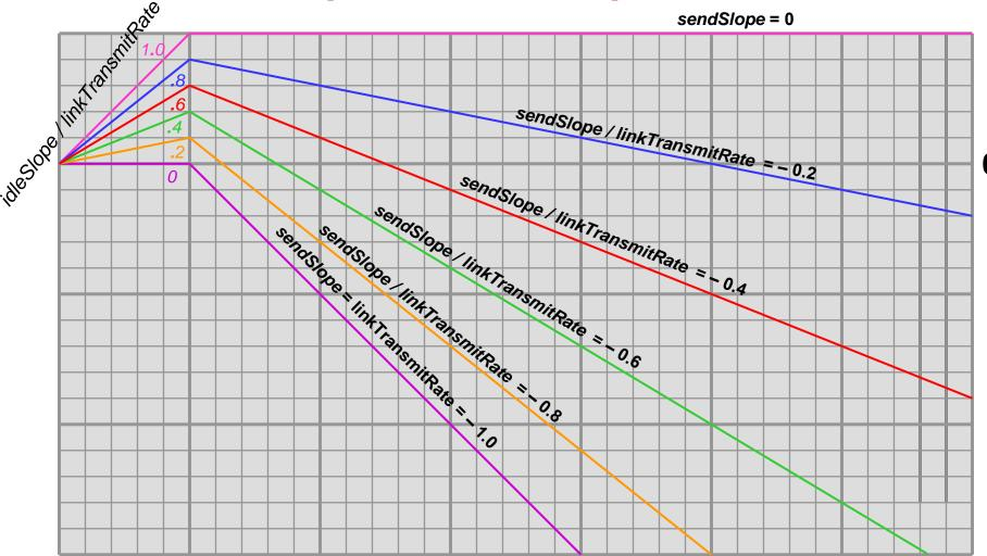
idleSlope / linkTransmitRate and sendSlope / linkTransmitRate for various data rates
