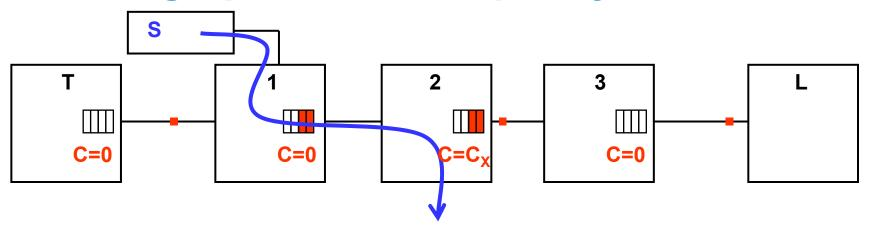
When the steady state is reached, we have two Bridges with permanently partially-full queues.
