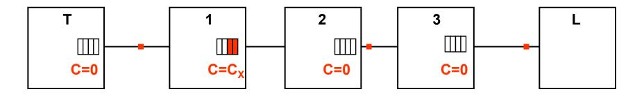
The new steady state is just as before, with all Bridges' credits hovering around 0, except that Bridge 1 has C<sub>X</sub> credit's worth of buffer filled up.
