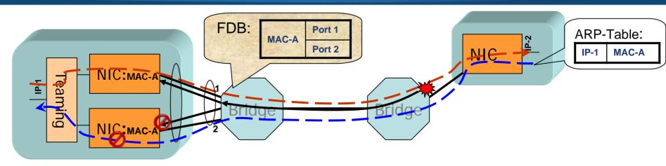
Flood CN packets on aggregated links to End Stations
