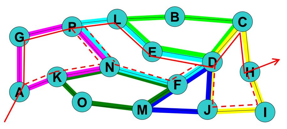
• The network designer or operator identifies cycles in the network topology in order to create the segments associated with an ESP.
