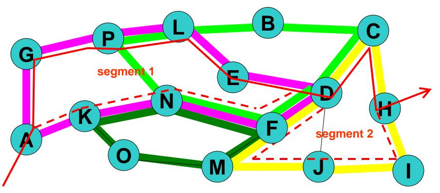
In the above figure, red ESP segment 1 is mapped to the violet cycle; red ESP segment 2 is mapped to the yellow cycle.
