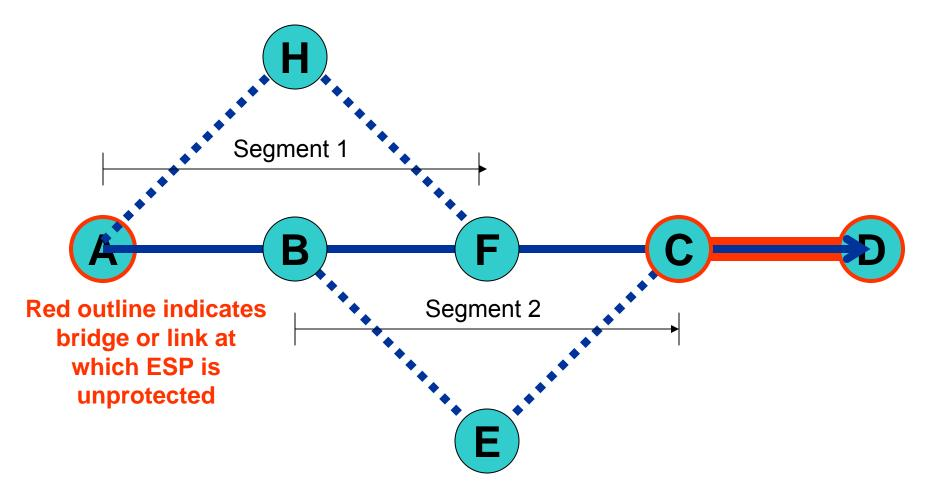
Segments can be defined such that some links and/or bridges in the interior of the ESP are not protected.
