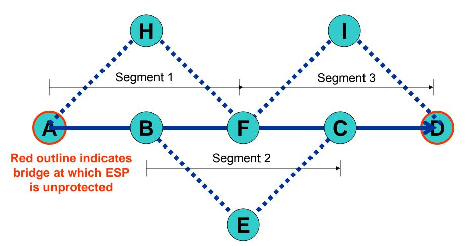
Segments can be defined to protect all links and bridges along the path of the ESP (excluding endpoint bridges)
