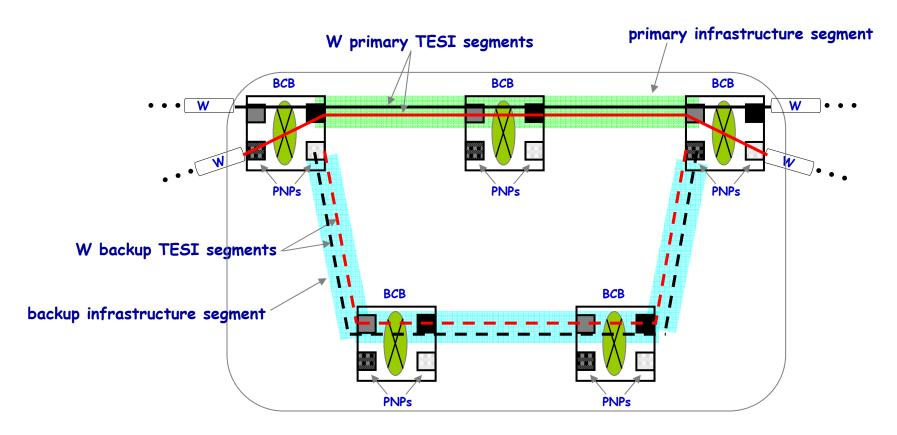
Multiple TESI segments can be associated with an infrastructure segment (two working TESIs shown in figure)
