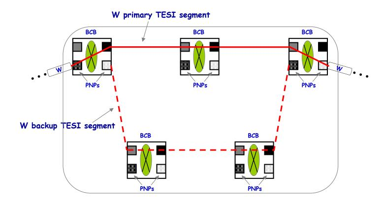
TESI Segment – Portion of a TESI bounded by a PNP at each end.
