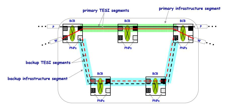
Multiple TESI segments can be associated with an infrastructure segment (one working and one protect TESI shown in figure)
