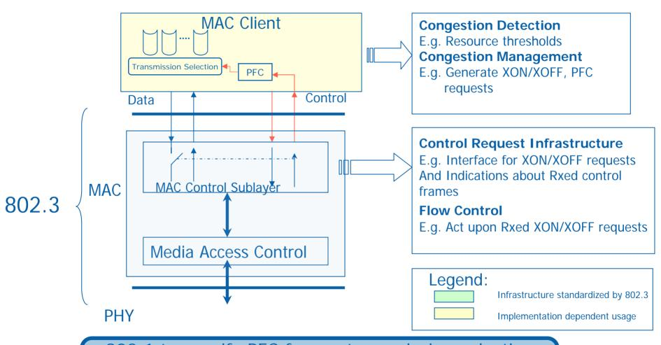
802.1 to specify PFC frame, transmission selection and control 802.3 maintains link FC frame and TS
