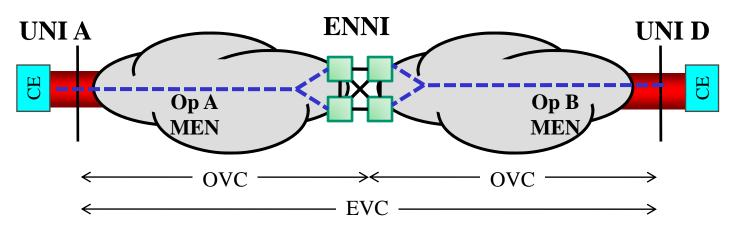
Does a redundant ENNI necessarily imply the E-line service be supported by a multipoint OVC? There are advantages to keeping the OVC point-to-point. Moderate advantages with Provider Bridge technology, but PBB incorporates significant optimizations for point-to-point Backbone Service Instances. (PBB-TE wouldn't support a multipoint EVC, but PBB-TE has it's own protection mechanisms.)
