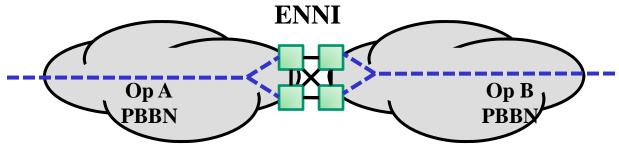
A similar, but more subtle, MAC address learning issue arises at a redundant PBB Peer ENNI. In a PBB network learning is based on a combination of B-SA and B-VID. The B-SA is the address of the I-component that encapsulated the packet. The assignment of I-SIDs to B-VLANs is local to each operator network.
