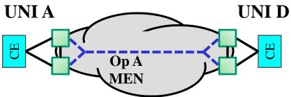
Generally assumed in carrier environment that load balancing will be done by VLAN. For the operator/provider, this is the S-VLAN. In other words both links between the CE and the provider may be active, but the provider will only transmit packets for any given S-VLAN on one of the links.
