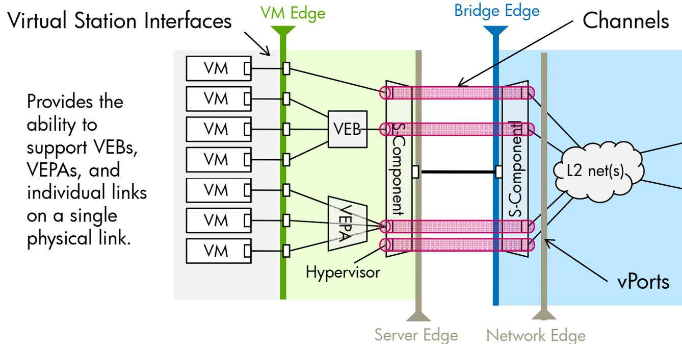
Provides the ability to support VEBs, VEPA, and individual links on a single physical link.
