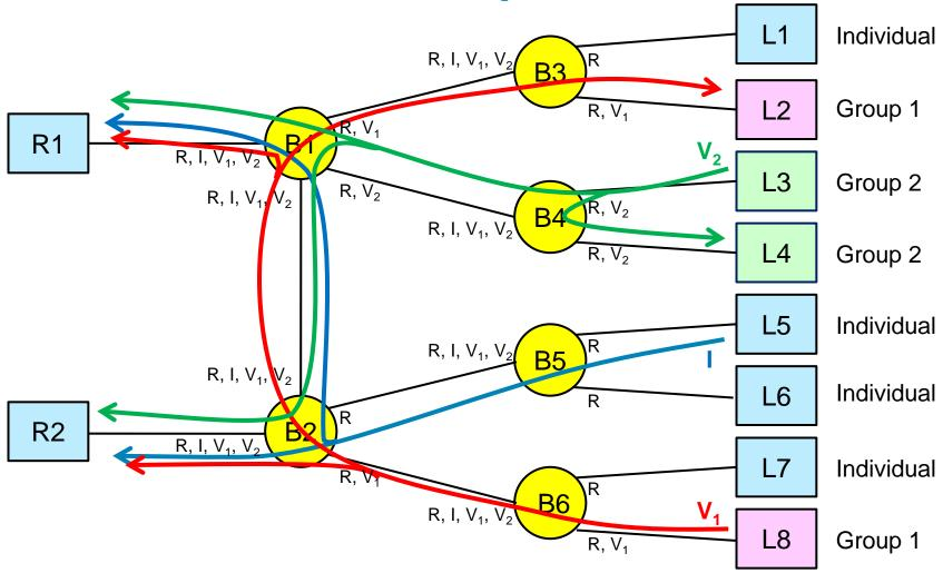
Each port marked with VLANs that can exit that port.
