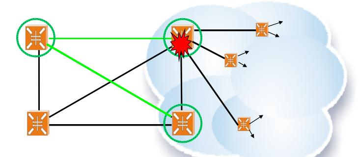
The TG is the node that conveys traffic from the network to the interconnected zone, and from the interconnected zone to the network.
