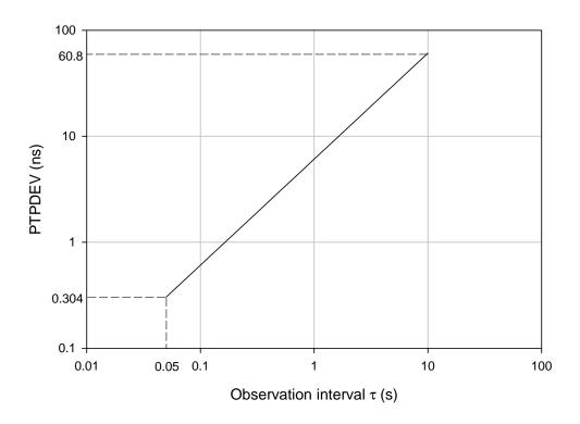
Figure B.3 – PTPDEV limit corresponding to wander generation requirement of Figure B.1 Formatted: Font: (Default) Arial, 10 pt, Bold
