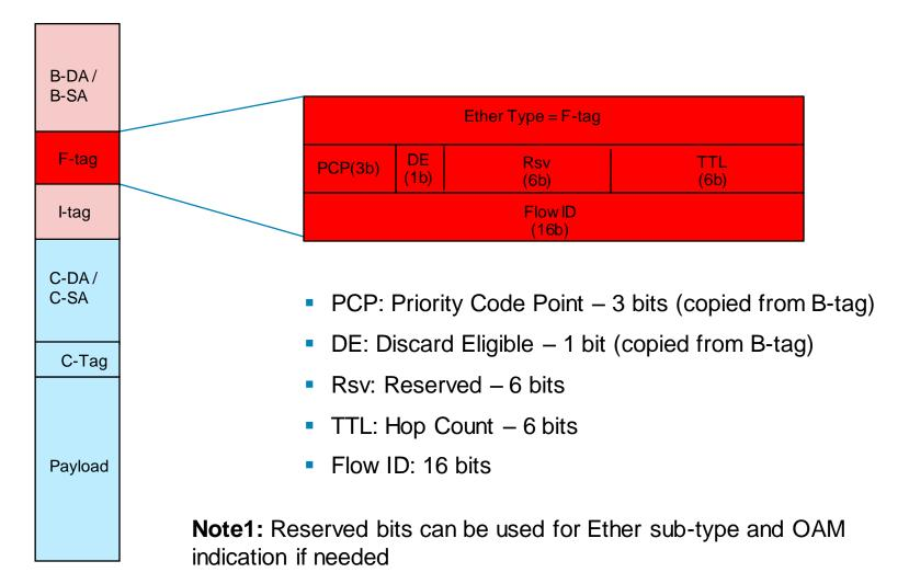
**Note2:** Only two additional bytes relative to 802.1ah frame. There is no need to send B-tag in the frame because unicast ECMP frames don't need B-VID. PCP/DE portion of B-tag is reflected in the F-tag.
