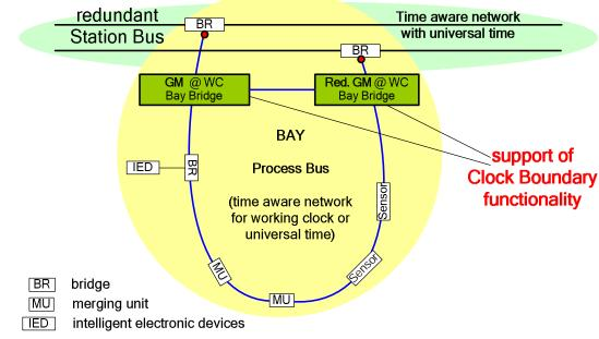
410 411 Clock boundary function makes slewing to second of universal time possible.
