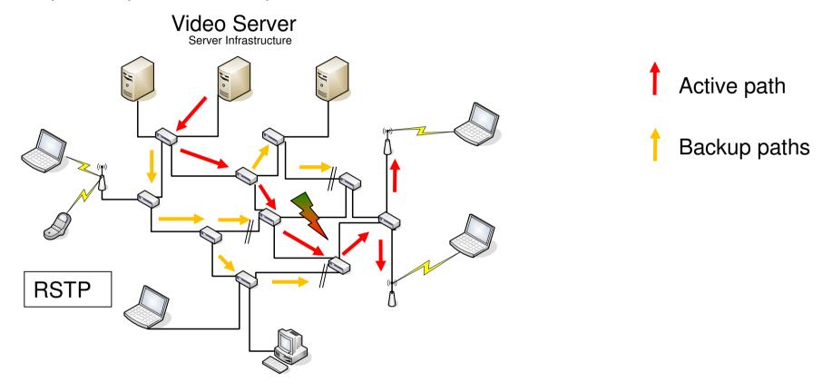
...after RSTP reconfiguration, a backup path takes over "seamlessly"
