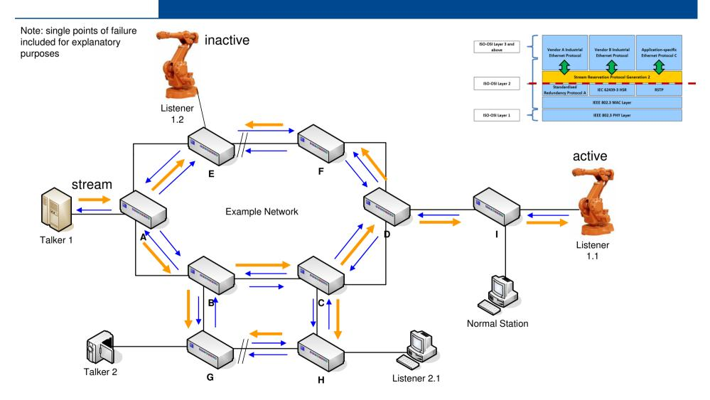
This effectively decouples Stream registration and transmission from the redundancy control protocol!
