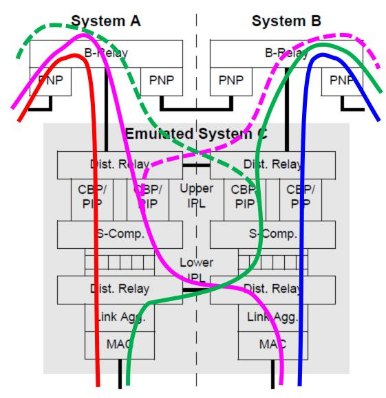
• If one expects far more failures at one end that at the other end (network end vs. LAG end), then one should arrange one's "criss-cross" CPBs to use the end that is expected to fail most often.
