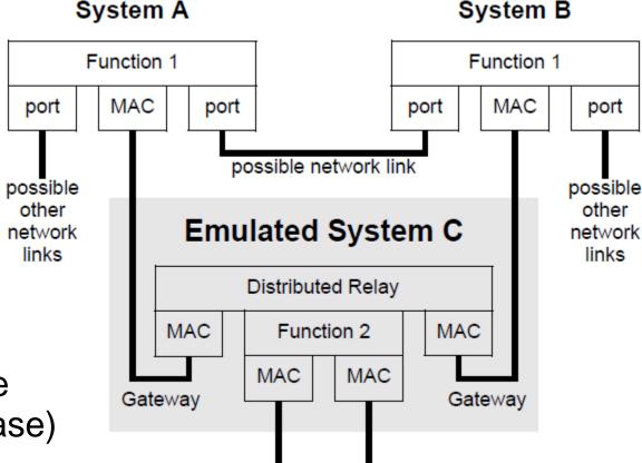
Two Systems visible above, with sole access from the network to a third (emulated) system with one or two down links, visible to Systems below.
