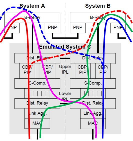
Similarly, a failure of a DRNI link or a movement of an S-VLAN to another DRNI link on the Left or Right CBPs does not generate any excess IPL bandwidth.
