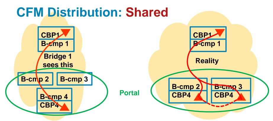
A TESI Up MEP (special I-TAG with no Customer addresses) is placed in a CBP that is distributed across two Portal Systems (some S-VLANs to one and some S-VLANs to the other). The two MEPs must look like one MEP, even for frame loss measurements.
