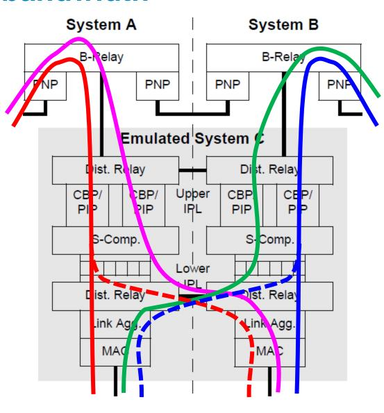
A failure at the "better" end of a criss-cross link actually improves the situation.
