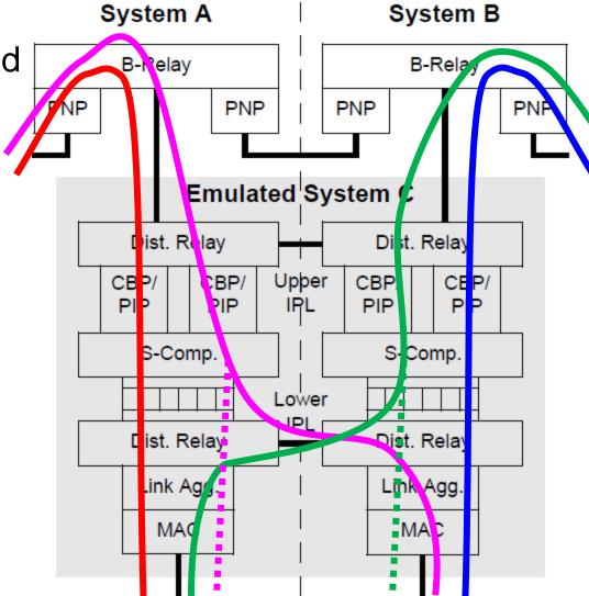
Only a failure at the "worse" end of a criss-cross link creates excess IPL bandwidth, in that frames in the failed service make two trips between the Portal Systems.
