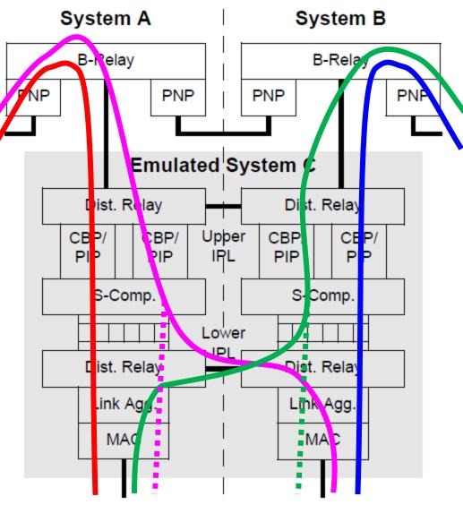
• If one expects far more failures at one end that at the other end (network end vs. LAG end), then one should arrange one's "criss-cross" CPBs to use the end that is expected to fail most often.
