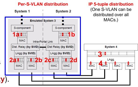
• Where do we put the Per-S-VLAN MEPs? In System 4, 802.1AX says that they must go in position 3. An implementation could reasonably place them in all four links (position 4), but the implementer must make sure that four MEPs emulate a single MEP.
