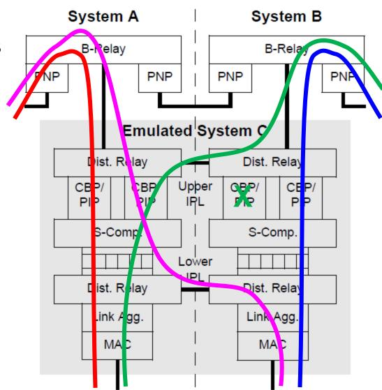
A failure of one of the (presumably many) ESPs in the Left or Right CBPs, would trigger the use of an alternate ESP that would use the Upper IPL.
