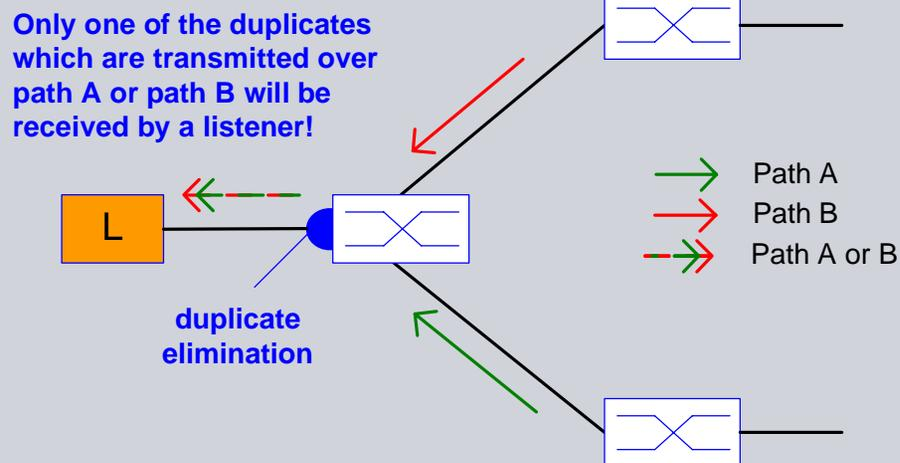
Frame path A received before frame path B
