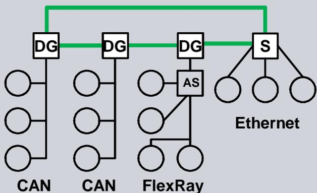
Parallel Networks for safety critical control applications
