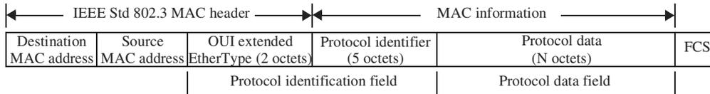
**Figure 13—IEEE Std 802.3 frame with the OUI Extended EtherType encoded in the Length/Type field**
