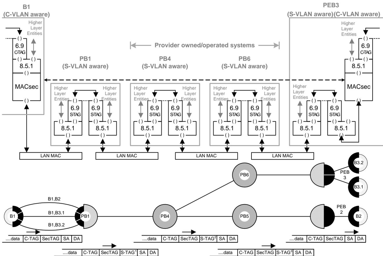
Figure 1—Interface stacks and paths for PBN tagged service interfaces
