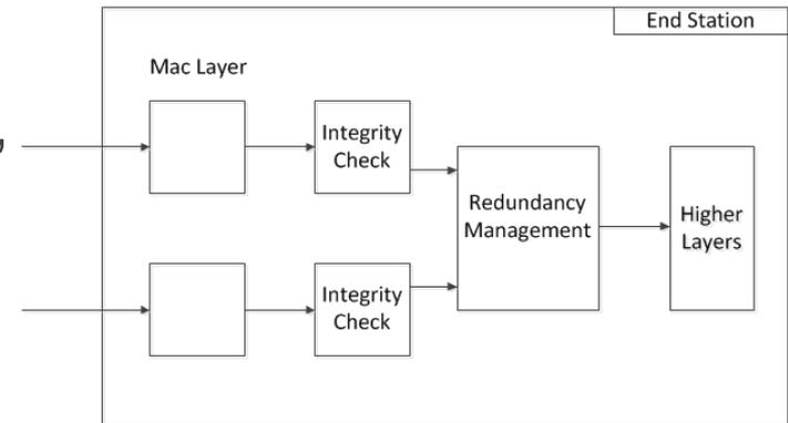
Integrity checking is used to identify whether the sequence number in a received frame is “plausible” i.e., within a configurable window (e.g., +1 or +2) higher than the sequence number in the previously received frame
