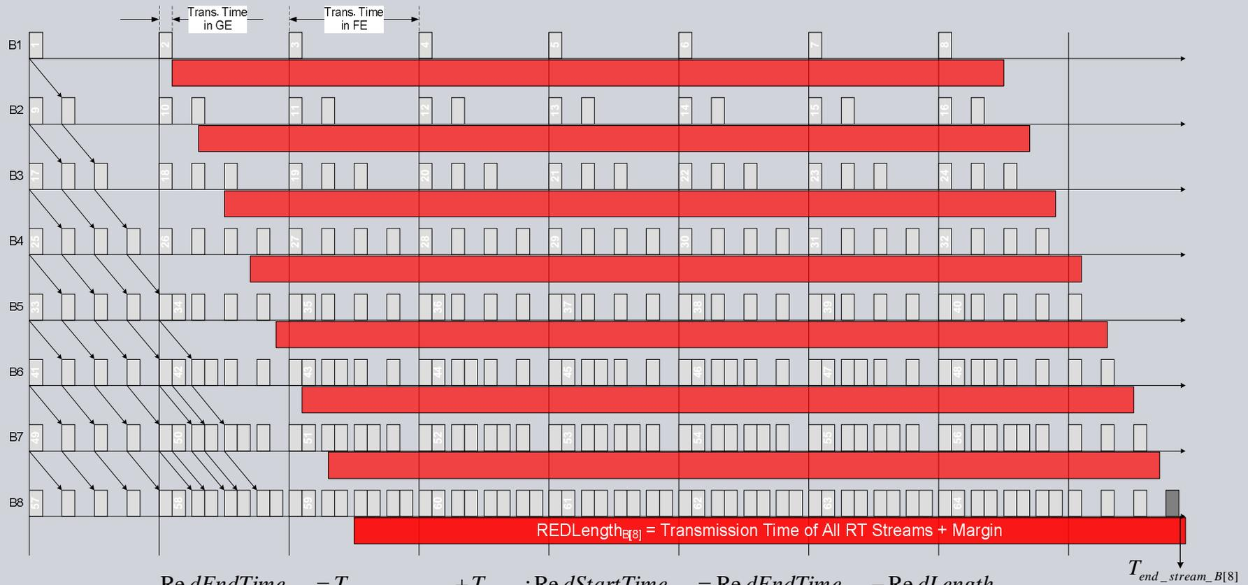
$$Re dEndTime_{B[8]} = T_{end\_stream\_B[8]} + T_{margin}; Re dStartTime_{B[8]} = Re dEndTime_{B[8]} - Re dLength_{B[8]}$$
