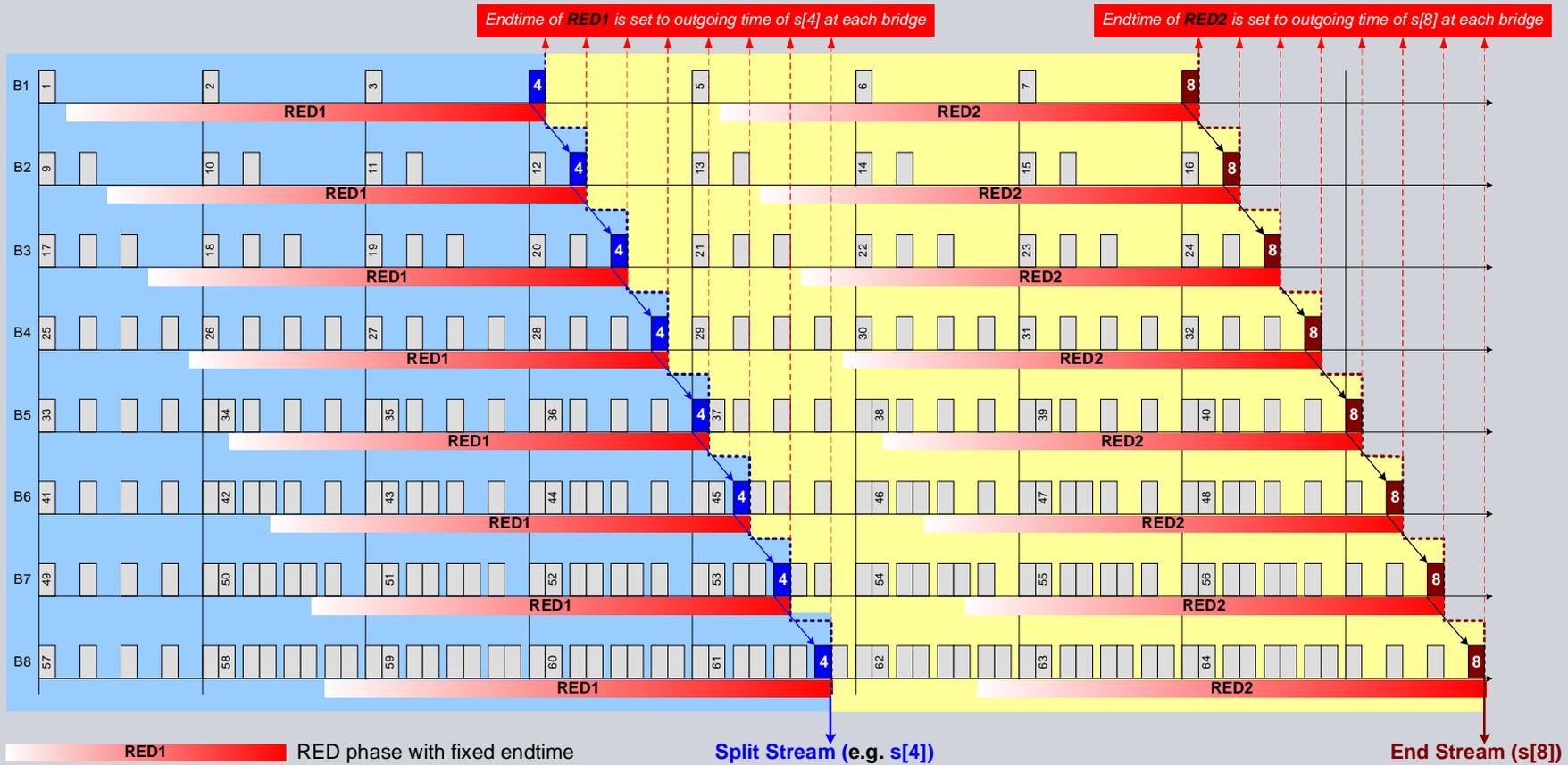
Step 1: locate a split stream (from farthest branch) and divide the RT transmissions into two segments (of similar loads)
