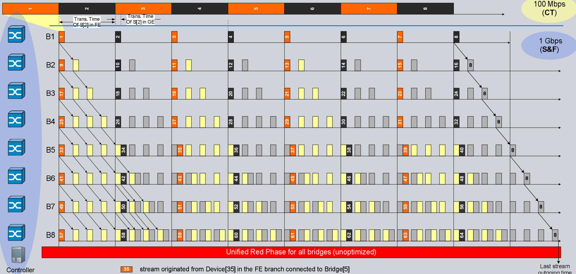
**Goal:** find a scheduling scheme splitting the long RED phase into e.g. two short ones for each bridge, in order to reduce bandwidth waste, while keeping worst-case latency (e.g. at stream[8]) unchanged.
