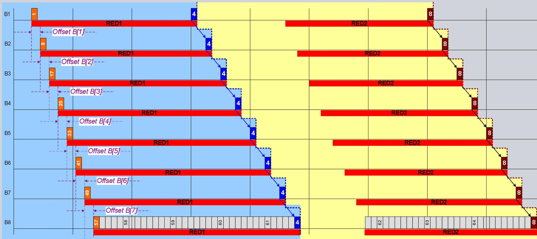
**Step 3:** determine RED phase starttime of last bridge (B[8]): set length of RED1/RED2 equal to the total transmission time of all streams that start before (incl.) split stream (S[4])/end stream (S[8])
