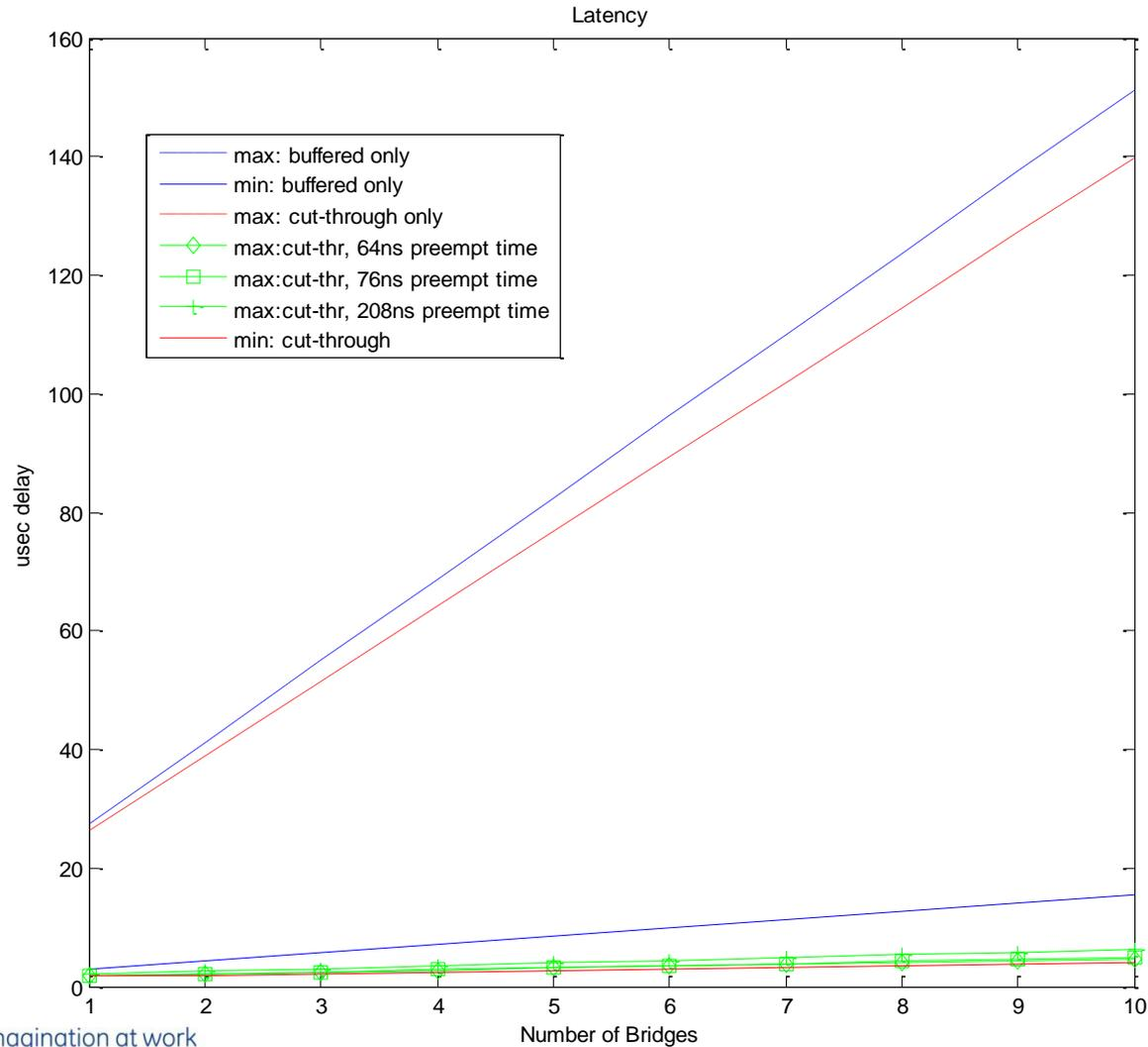
From xmit bit on edge node to last recv bit on edge node.
