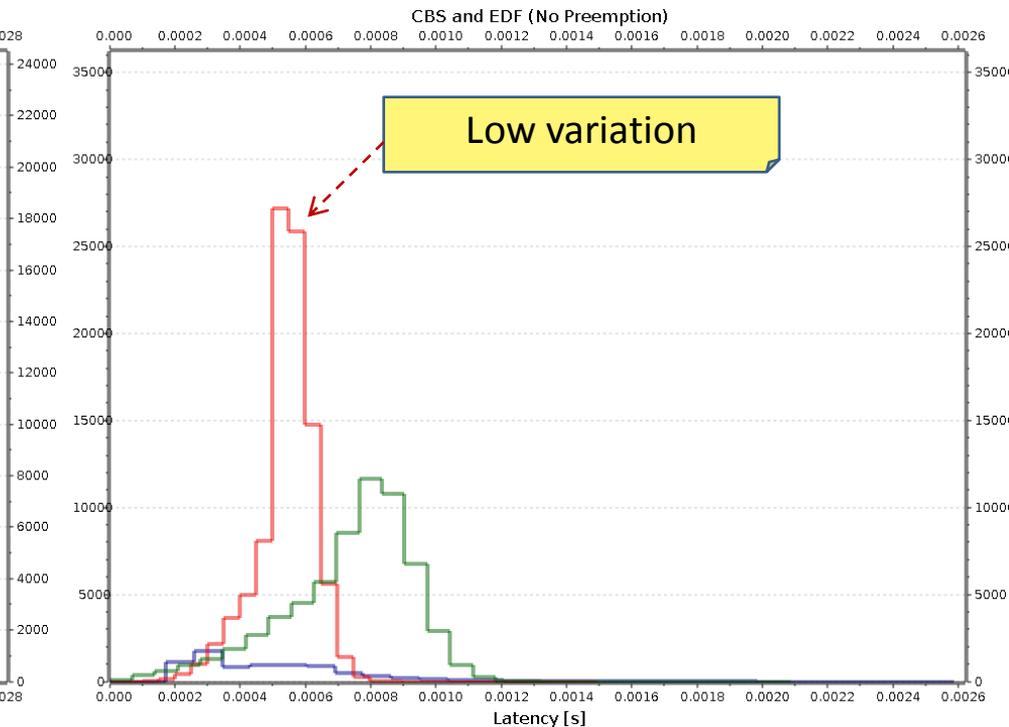
X-Axis: Latency in seconds, Y-Axis: Number of frames.
