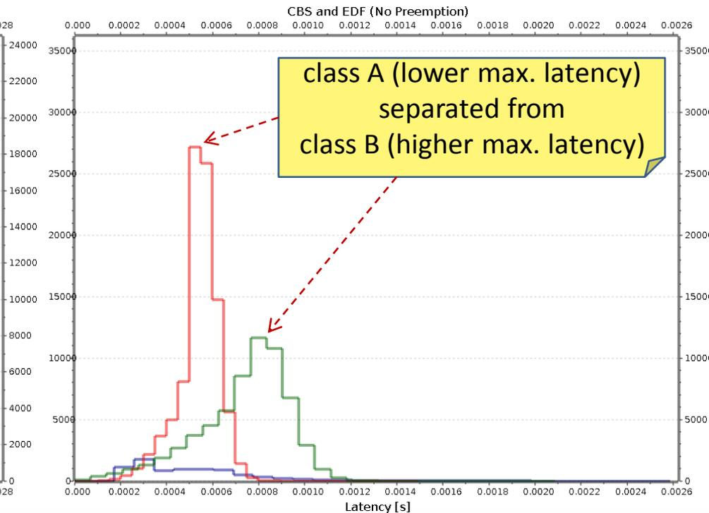
X-Axis: Latency in seconds, Y-Axis: Number of frames.
