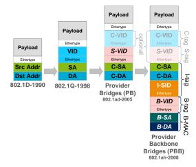
Fig. 4. Encapsulation formats provided by Ethernet
