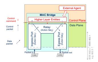
Fig. 2. Bridge architecture
