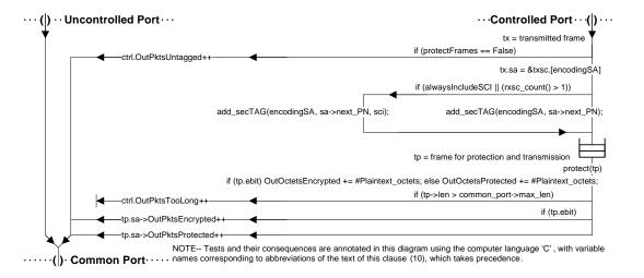
Figure 2—MACsec transmit processing
