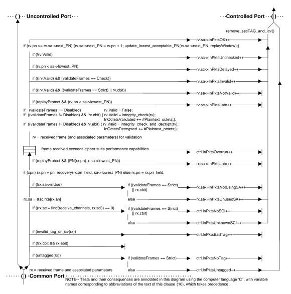
Figure 1—MACsec receive processing (.1AE-2006 amended by .1AEbw-2013)
