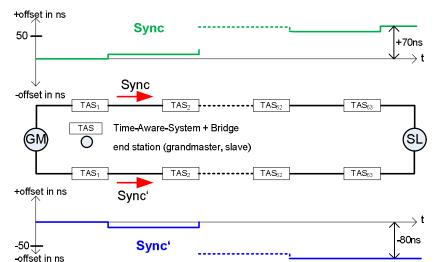
Example for deviation between GM time (distributed over redundant Sync messages) and Slave local synchronized time
