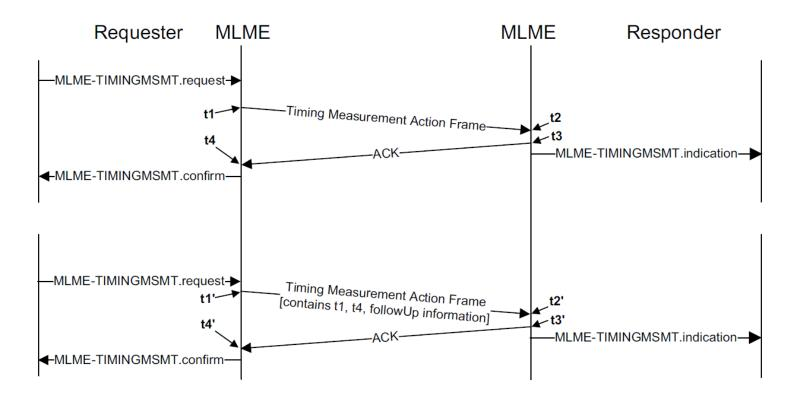
Figure 12-1—Timing measurement procedure for IEEE 802.11 links
