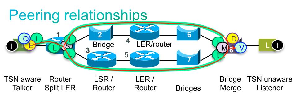
A network of Label Switched Paths (LSPs) connects E to S to M to D. Each endpoint is a Label Edge Router (LER) function.
