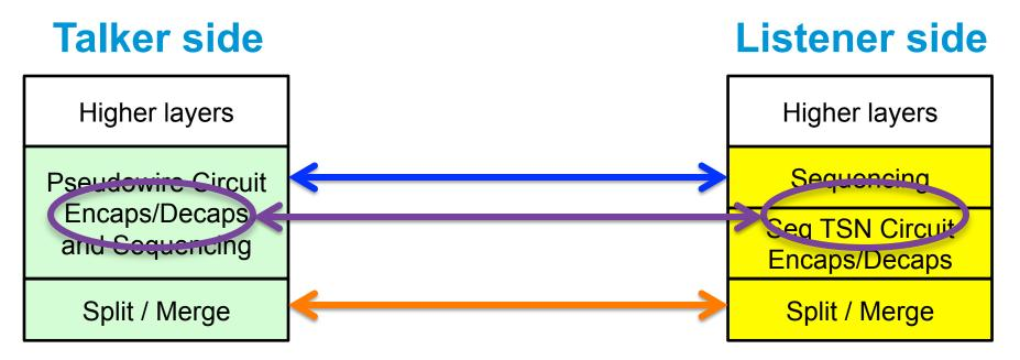
Because the sequence numbers are similar (preferably, the same!), the Split/Merge functions have no tag layer, and we choose to have no other layer between the TSN Circuit ID and Sequencing layers, ....
