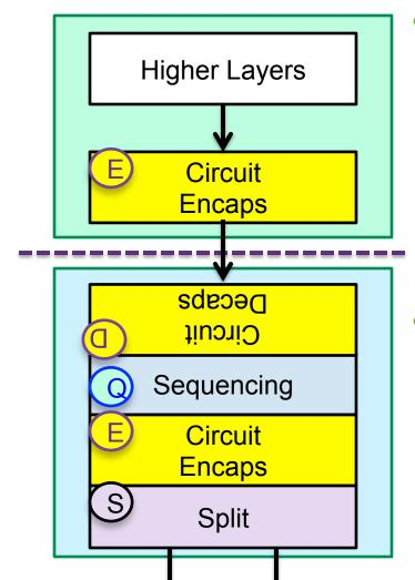
In this example, the Circuit Encaps is in the Talker system (above the link).
