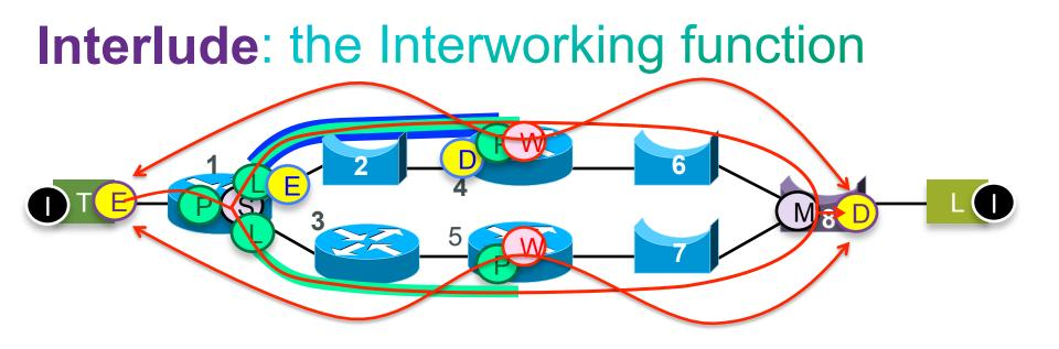
The Interworking Functions () enable the TSN Circuit Encaps function () and the Decaps function () at the very ends of the network to be peers, just like the Ethernet end-to-end case.
