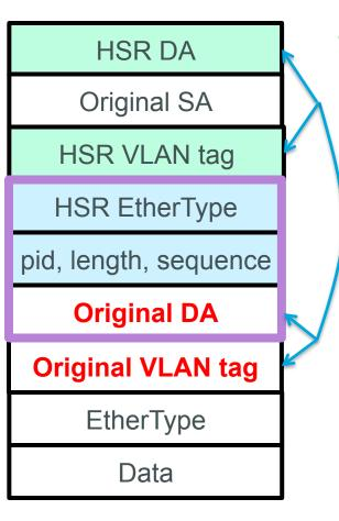
At first glance, the fact that HSR encapsulates the original Destination MAC address and VLAN tag seems attractive, because the decapsulation function can restore the original frame using data in the frame, instead of relying on stored information provided by the control plane.
