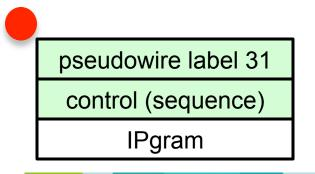
Instead of using an interworking function, we can carry the pseudowire along using the normal MPLS Ethernet encapsulation.
