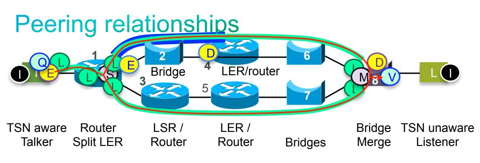
An extra TSN Circuit Encaps/Decaps pair is needed to convey the circuit over the Bridged LAN represented by Bridge 2.
