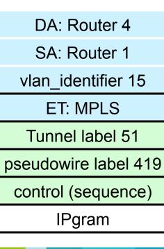
The upper tunnel would have look like this, on the wire, when labeled with Tunnel 51, except that ...
