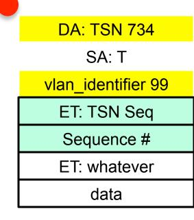
The Sequencing function adds a new TSN sequence number tag, to be defined by IEEE 802.1.
