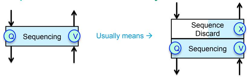
To prevent clutter, unless otherwise noted, the sequencing removal action (v) will usually imply the Sequence Discard sublayer (x) in this deck.
