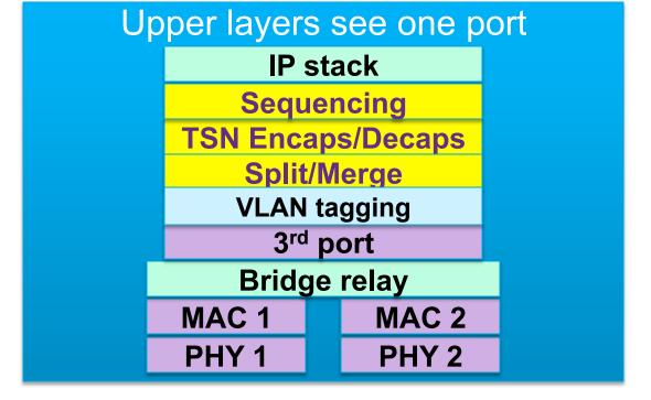
In the preceding diagram, the Split/Merge function is assumed to alter the circuit\_identifiers of the two streams, and generate two frames, each with a different encapsulation, so that the Bridge can send those frames on the other two Bridge Ports.
