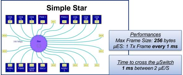
**200 μs** for μES to μES/AFDX<sup>®</sup> **100 μs** for AFDX<sup>®</sup> to μES
