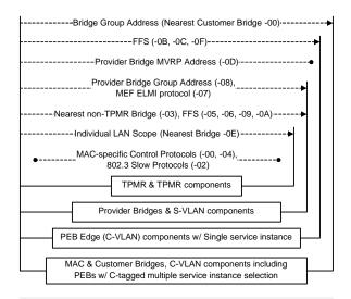
802.1Q Reserved addresses are the block of 16 beginning 01-80-C2-00-00-00 Addresses (inc. -07) are not assigned for the exclusive use of particular protocols. EtherTypes are required as other protocols can use each address, with possible constraints (e.g. for -02).
