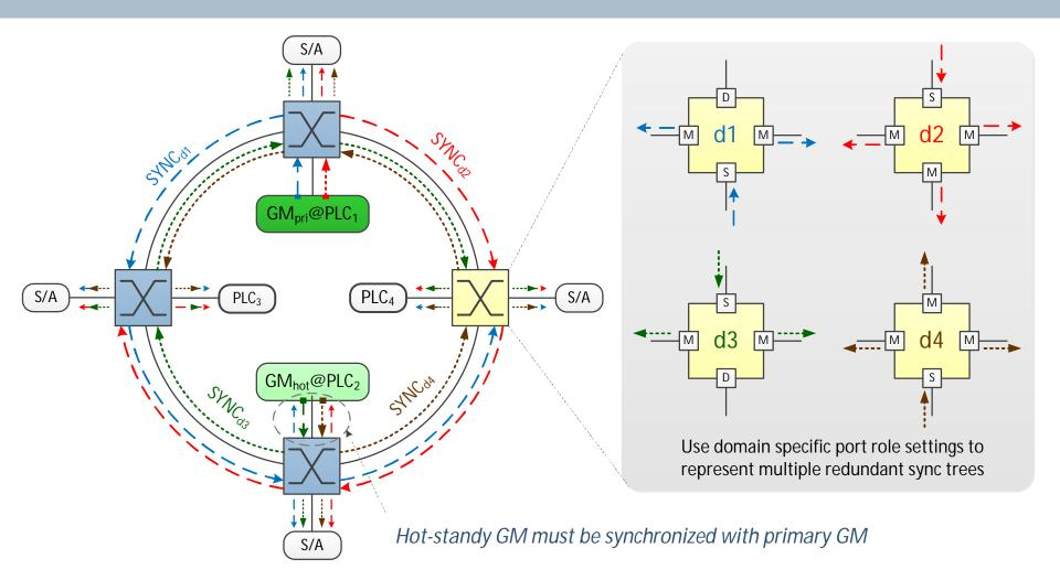
One primary GM and one hot-standby GM with four Sync trees in four gPTP domains (d1, d2, d3 and d4)
