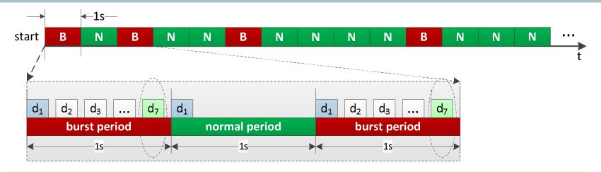
avg. propagation delay in the burst period is calculated at the end of each burst period by \*  $D_{ava} = avg(d_1, d_2, ..., d_7)$
