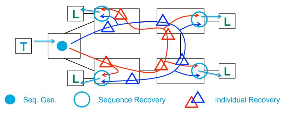
Each Listener gets only one copy. Packets are not discarded until just before output to the Listeners, so that latent errors can be detected.
