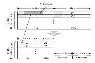
I/Q bit-width 8 bits UL and 10 bits DL here is just an example and the actual bit-width needs to be determined carefully by simulation and empirical studies.
