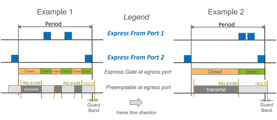
Guard band can protect the express traffic completely from interference from preemptable traffic
