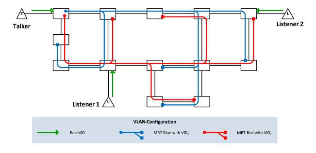
Figure 8 - Example VLAN configuration for ladder redundancy
