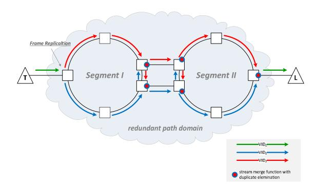
Figure 7 - FRER for ladder redundancy
