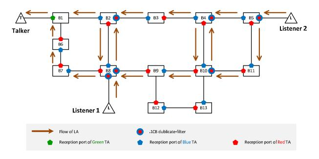
Figure 10 - RAP Listener attribute propagation for ladder redundancy
