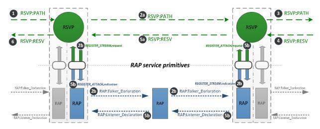
Figure 12 - Parallel operation of RSVP and RAP within a L2 sub-network
