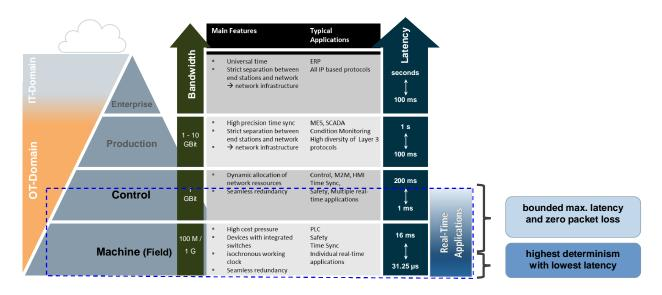
Figure 1 - Industrial real-time applications on the classical automation pyramid
