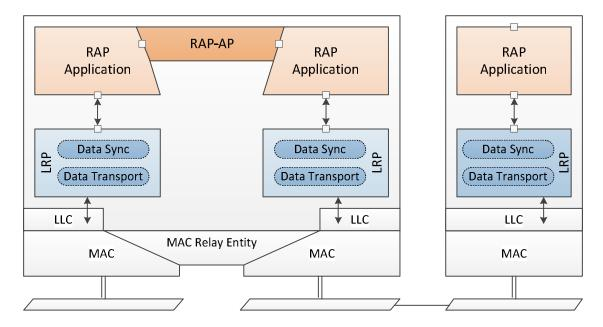
Figure 2 - Architecture of RAP on a Bridge and an end station
