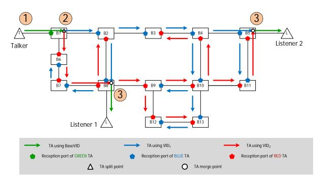
Figure 9 - RAP Talker attribute propagation for ladder redundancy
