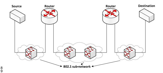
Figure 11 – A DetNet domain containing L2 sub-networks
