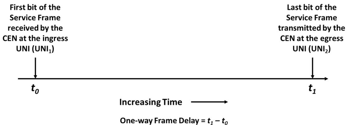
Figure 16 – One-way Frame Delay for Service Frame
