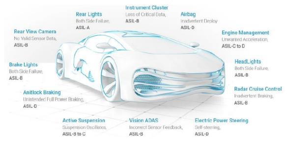
Figure 8 – Example ASIL Assignments in a Car<sup>10</sup>
