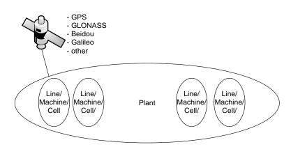
Figure 23 – plant wide time synchronization
