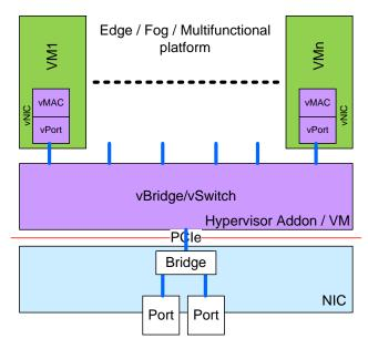
Figure 15 - Ethernet interconnect with VM based vBridge
