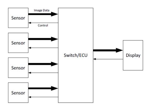
Figure 6 – Examples of an Asymmetrical Ethernet Links
