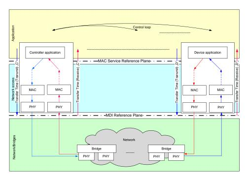
Figure 26 - Principle data flow of control loop
