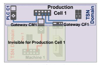
Figure 22 – Gateways with two TSN domains and an attached Fieldbus
