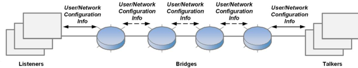
Figure 46-1 — Fully Distributed Model
