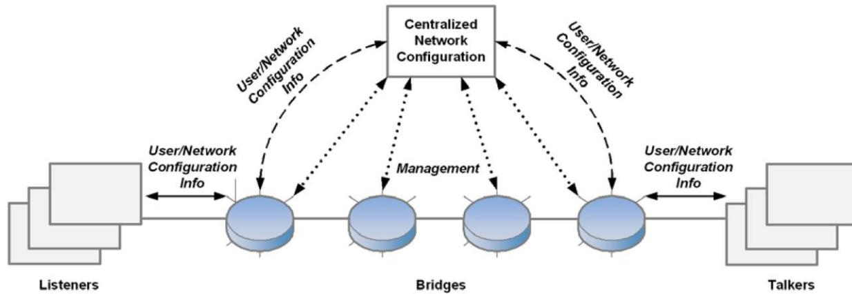
Figure 46-2 — Centralized Network / Distributed User Model
