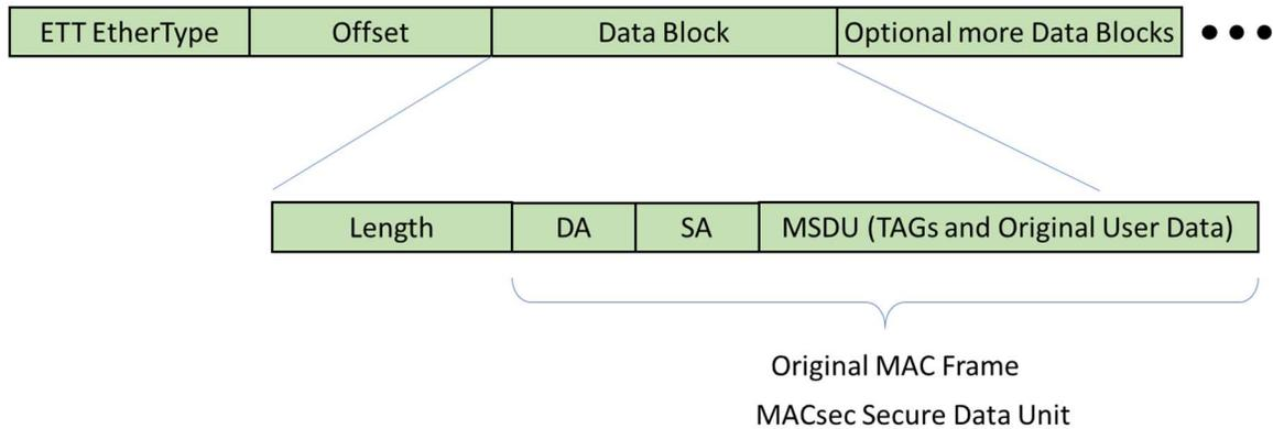
Figure 4 Proposed Logical format of MAC Tunnel Data Unit (MTDU)
