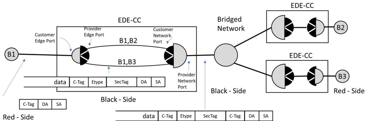
Figure 1 Existing MACsec between Ethernet Encryption devices
