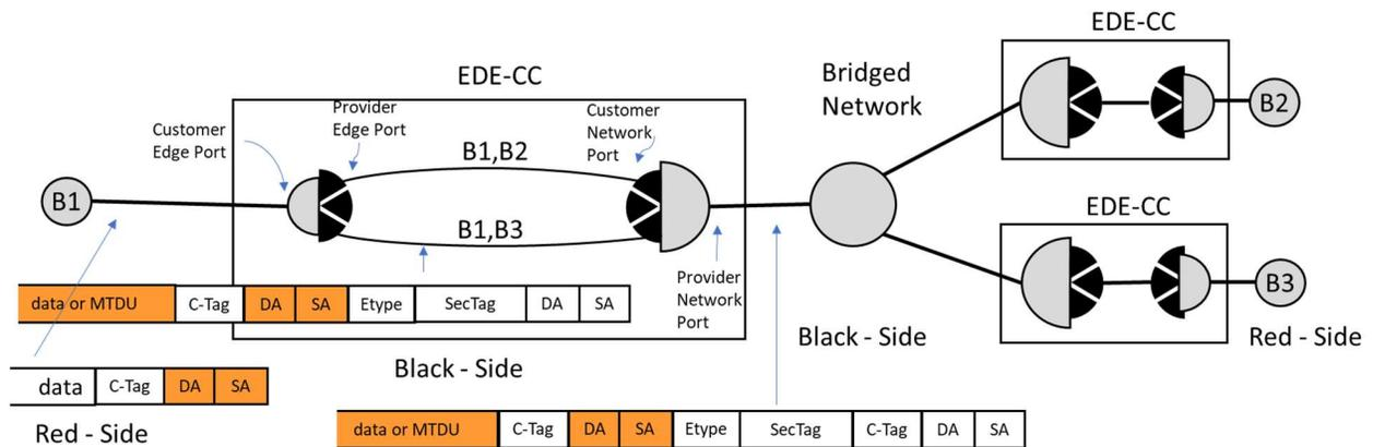
Figure 2 Example Tunnels between Ethernet Encryption devices with E-TFS
