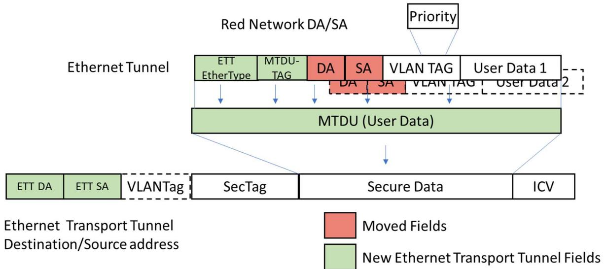
Figure 3: Proposed Ethernet Traffic Tunnel Functional Diagram
