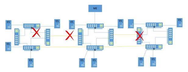
Figure 8: Coupled rings topology – multiple faults
