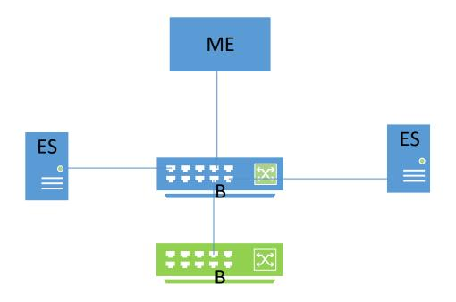
Figure 3: Simple TSN Domain – plug a Bridge
