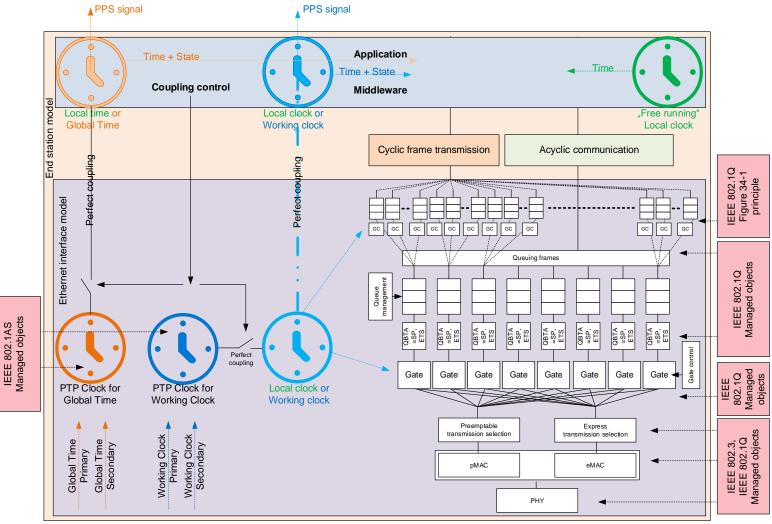
The end station interface and end station model needs to include synchronization.
