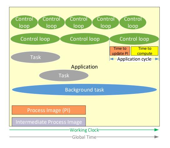
Background task, Time event task and Control loop tasks are started time triggered.
