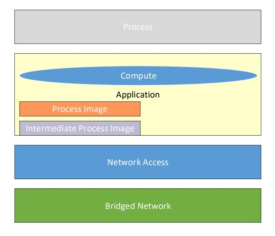
Nowadays, the process image has a size from less than 1k Bytes up to 1M Byte.
