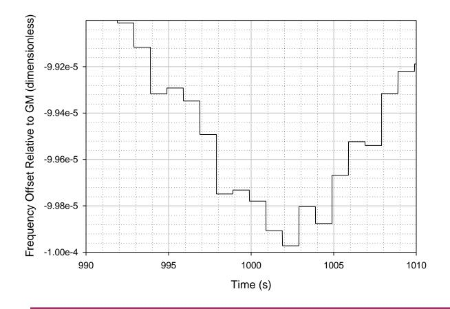
Detail of 100 – 102 s. Jumps reflect errors in neighborRateRatio measurements due to timestamp granularity, at each of the 100 Nodes.
