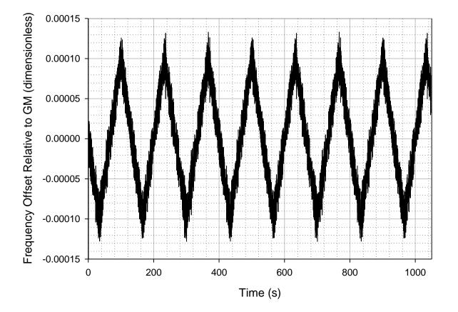
Case 6s, PTP Instance (node) 20 Frequency offset relative to GM Clock Model: Triangular wave phase and freqeuncy error variation, with zero phase offset of this variation at each node)
