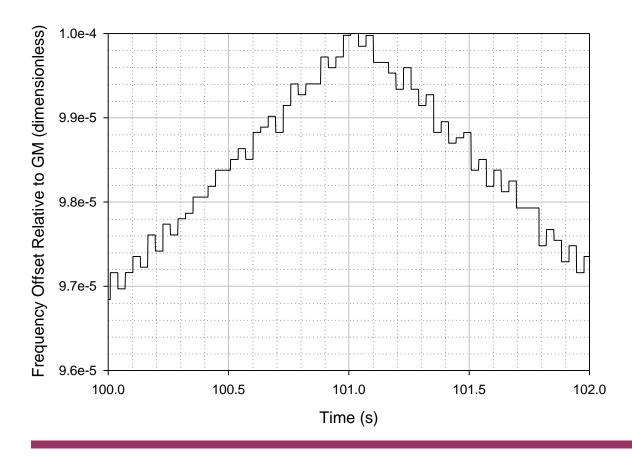
Detail of 100 – 102 s. Jumps reflect errors in neighborRateRatio measurements due to timestamp granularity, at each of the 100 Nodes.
