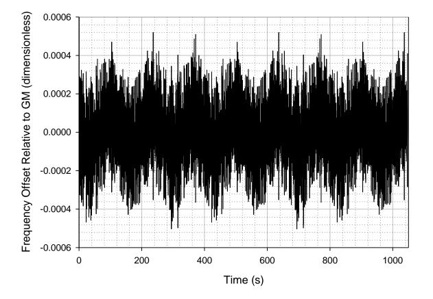
Case 6s, PTP Instance (node) 30 Frequency offset relative to GM Clock Model: Triangular wave phase and freqeuncy error variation, with zero phase offset of this variation at each node)
