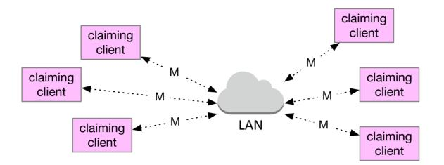
Per P802.1CQ/D0.5, N clients send claim messages to claiming multicast address M
