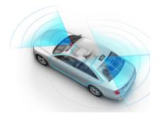
~ 10ms E2E network latency required to avoid collision based on 3 – 27 Mbps application signal rate
