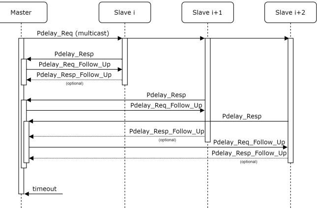
"Slave i+n" simply demonstrate how responses to Pdelay\_Req of multiple ports can overlap. Pdelay\_Resp\_Follow\_Up is optional, if the slave port will never change its role to a master port. A 10Base-T1S slave node will most likely never be a GM instance, as long as there is a 100Base or faster network connected, for better clock quality. But distribution direction can change, i.e. in case of redundant network paths.
