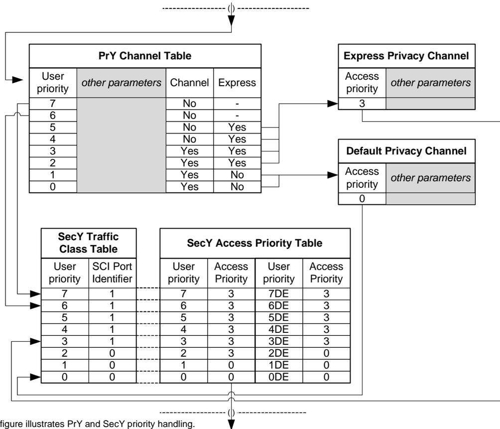
This figure illustrates PrY and SecY priority handling. It is not a recommendation for a default configuration.
