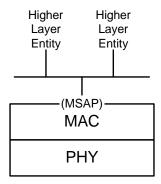
Each 'Higher Layer Entity' at the same MSAP fills in/recognizes its protocol identifier in initial MSDU octets.
