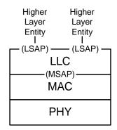
Each 'Higher Layer Entity' connects to an LSAP that adds/recognizes/removes its protocol id from the MSDU octets.
