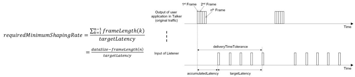
Figure Z-4— Frame propagation within delivery time tolerance while minimizing over-provision of bandwidth reservation
