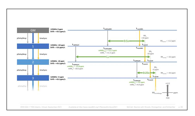
Note that a GM Clock Drift has a similar effect as in the simple analysis: it pushes every subsequent Rate Ratio measurement off in one direction, but in this case the effect is amplified by the initial delay between mNRR<sub>1GM</sub>.
