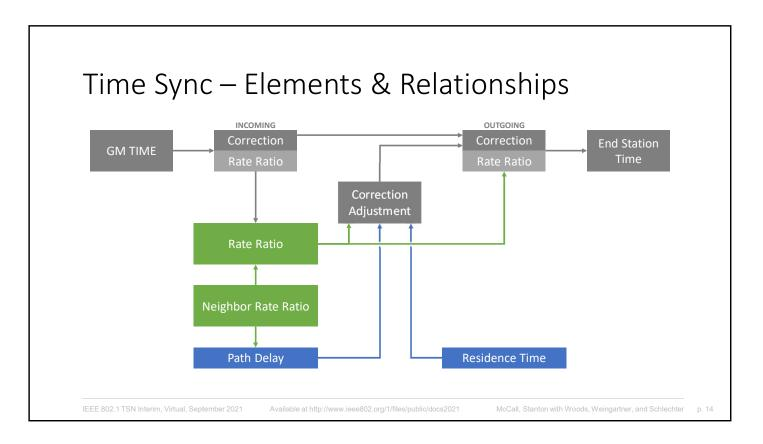
At each bridge there is a process for taking the incoming Correction Field and Rate Ratio and adding effects of the local pDelay (between the local and upstream device) and Residence Time.
