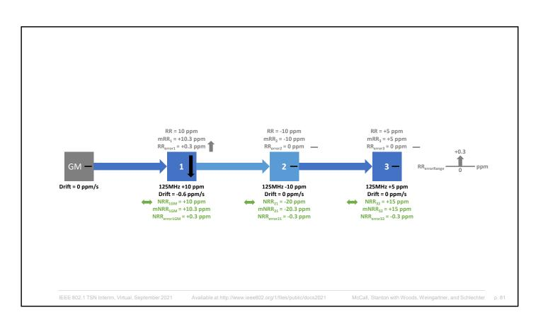
Simple in that...if you feed NRR directly into RR, and don't account for time between measuring mNRR and using mNRR, i.e. applying it to Rate Ratio.
