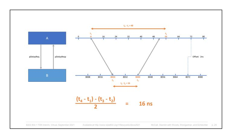
At an offset >2ns, the measurement is no longer 16ns...
