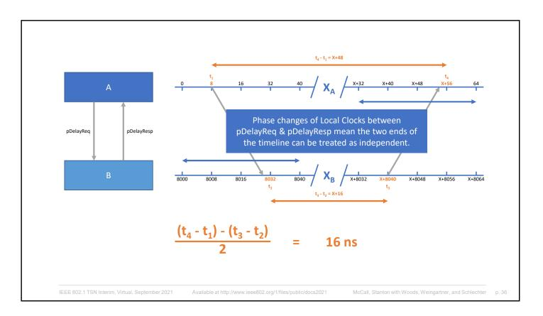
Because the left and right ends of the timeline can effectively be decoupled from each other...because there are different numbers of clock ticks in  $X_A$  and  $X_B$  (which is compensated for by NRR...which we aren't not currently considering)...you can look at the measurement probabilistically...which looks like this...
