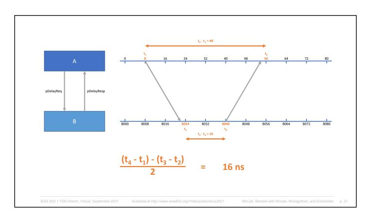
8ns is our Timestamp Granularity...which means the pDelay Req could arrive at any time between clock ticks and the Timestamp will actually reflect the next clock tick.
